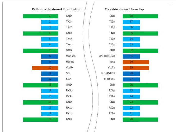
Figure 2 QSFP112 Module Contact Assignment
