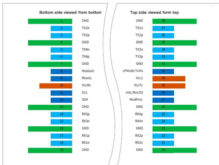
Figure 1 QSFP112 Module Contact Assignment
