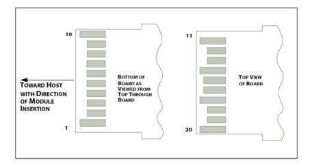
Figure 2 SFP28(56) Module Contact Assignment
