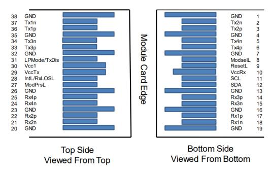
Figure 1 QSFP28(56) Module Contact Assignment
