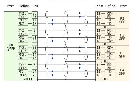
Figure 3 QSFP28(56) to 4\*SFP28(56) Direct Attached Cable Assembly Wiring
