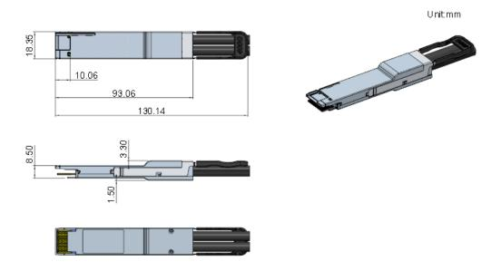
Figure 5 QSFP-DD Form Factor
