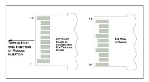
Figure 2 SFP28(56) Module Contact Assignment
