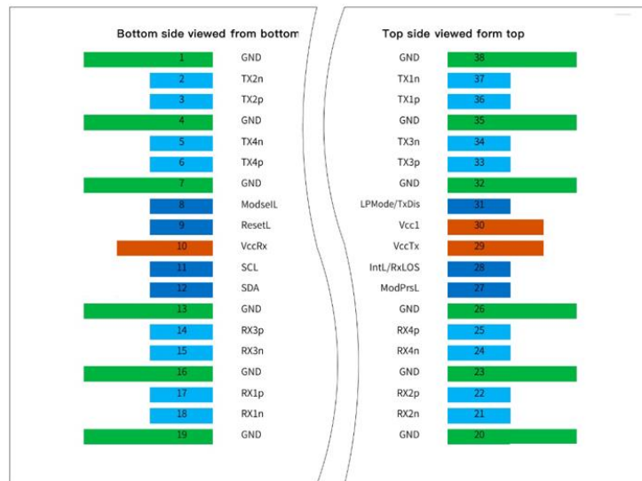
Figure 2 QSFP112 Module Contact Assignment
