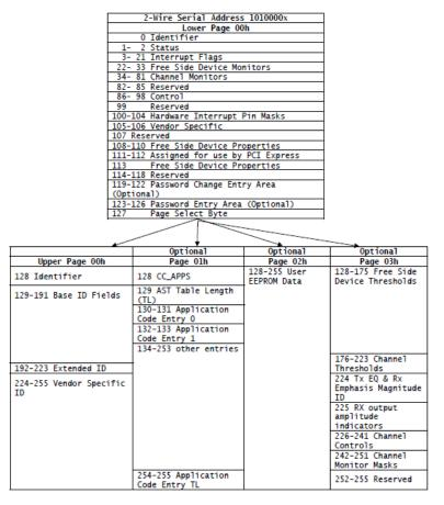
Figure 2 - Two-Wire Interface Fields
