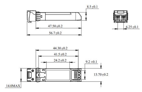
**Figure 3 - Mechanical Specifications**
